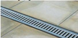
Single skin removable drain grating, made of 16 swg. Ss, with perforations of 15 mm wide, spaced 25 mm apart from each other, laser cut to a uniform finish. Width of grating shall be 150 mm, with a rest of 25 mm. Length to be 1200 mm
