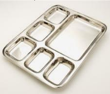
Made of 24 swg 202 grade steel, overall dimensions not less than 450x350 with indentations of not less than 20mm. Edges to be double folded inwards and the unit to be buffed to a shining finish.
