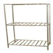
Overall dimensions of 1200x750x1900 height. Frame to be made of 14 swg 38 mm dia ss tubes, fitted with adjustable ss bullets. In all, three partitions to be made across the height, equally distributed, with lowest shelf at 150 from bottom. Shelves to be fabricated of 16 swg 25 mm dia ss tubes, welded to the frame across the length, at intervals of 150 center to center.
