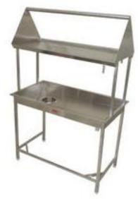
Overall dimensions of 750x750x850. Top to be recessed by 50 mm on a 25 mm radius at edge, and be provided with a 200 dia garbage chute, fabricated of ss, extending by 150 under the top. Bottom framework should be so designed as to facilitate movement of garbage bin. One overhead crate shelf to be provided, made of 25 dia ss tube frame and a 16 swg flat, fitted 750 above the top.
