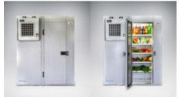
Model Pre Serva of RINAC make, compact reach in chiller, overall dimensions of 1800wx1200dx2100h, 3500 lrs (200 kgs) volume, 60 mm thick PUF insulated panels, clear door opening of 600x1800, delivering a temperature of +2 to + 8 degree celcius, operating on 220v/50Hz/1Ph power input with a consumption of 1265W. Inside to have adjustable Cambro shelving system.
