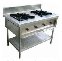
Overall dimensions of 1200x750x850. Top to have one each of T-22 and T-35 burners, housed properly in a suitable ms frame, with pilot lamps, internal gas piping, wire braided pig tails, gas flow regulators, and each burner to have a 500x500 heavy duty cast iron vessel rest rated for 20 kgs per square foot. Legs to be of 38 mm dia 16 swg ss pipes, fitted with adjustable ss bullet feet. Bottom frame of cross bracings made by 25 mm dia 16 swg ss pipes welded at 150 intervals, 150 above floor level.
