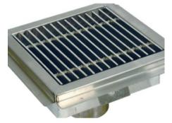
Overall dimensions of outer frame to be 600x600x100 mm deep. Unit to be made as a two part system, with outer frame to be made of 16 swg ss. Sheet, machine cut and machine bent for accuracy. The removable part to be made of 3 mm thick ss 304 grade sheet of 25 mm thickness,
