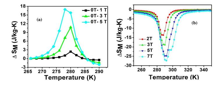
Variation of magnetic entropy with temperature of (a) Ni-Mn-Sn Heusler alloy doped with B (b) Mn-Fe-P-Si alloy
