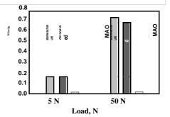
Superior abrasive wear performance of MAO coatings as against the hard anodized coatings against silica abrasive as per
