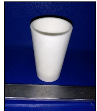
Green SiAlON crucible produced by gelcasting technique at ARCI
