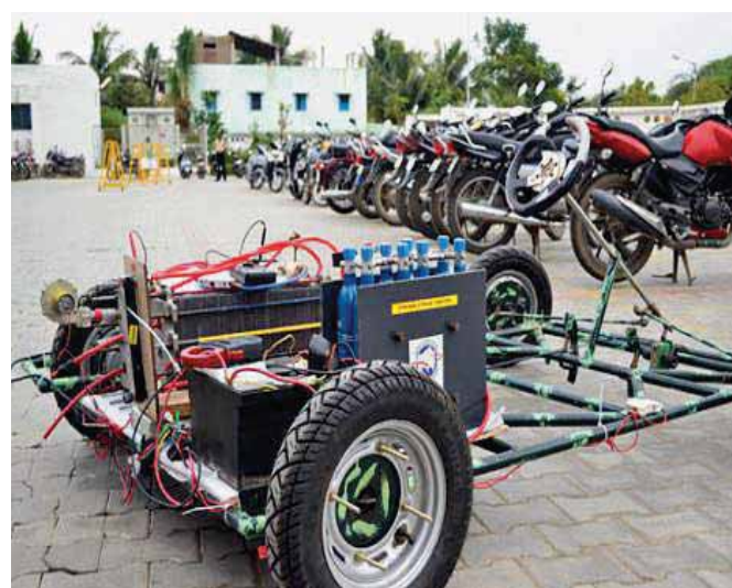
Go-Kart with 1 kW PEM fuel cell stack
