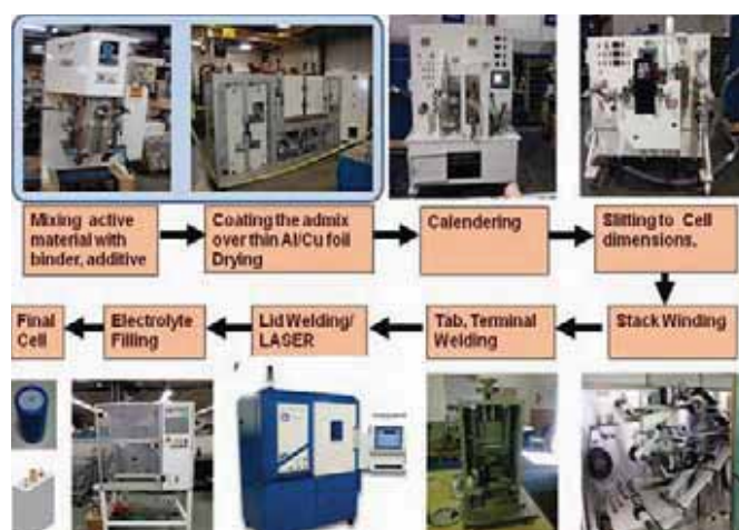
Scheme 1: Process for manufacturing LIB
