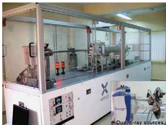
Fig. 1 Dual source (Cr & Mo) SAXS system installed at ARCI. Inset shows the assembly of dual sources (Cr and Mo) on a moving stage
