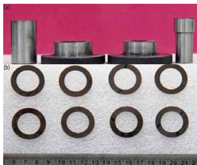
Fig. 1 a) Die fabricated for punching out toroid shaped rings and b) typical Fe-P rings used for AC magnetic measurements
