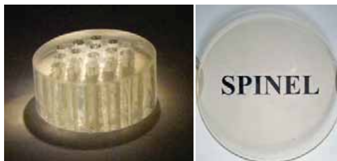
Fig. 1 Photographs of transparent (a) honeycomb and (b) flat sample
