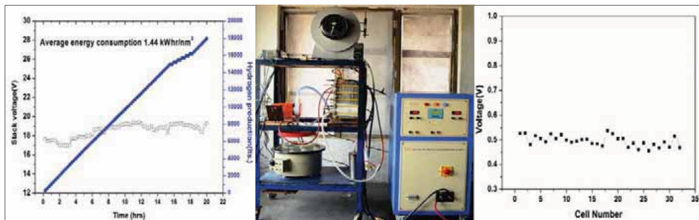
1000 l/hr PEM based Hydrogen generator and performance data
