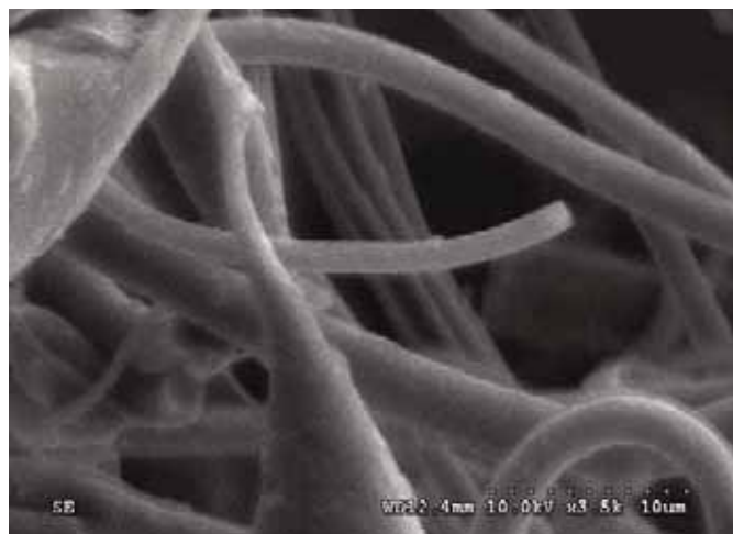
Fig. 1 FESEM image of MWCNT-Carbon nano-fiber composite
