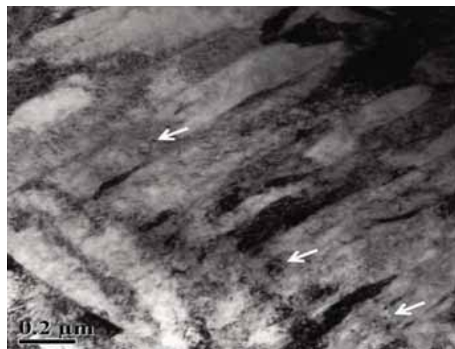
Fig. 1 Bright field TEM image of laser treated H13 tool steel with laser specific energy of 62 J/mm 2
