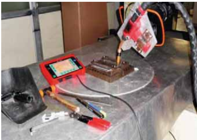
Fig. 1 Experimental set-up for joining studies using CMT process
