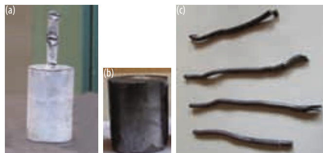
Fig. 2 (a) Vacuum sealed MS can (b) forged billet and (c) extruded rods
