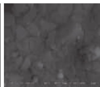
Fig. 3 Representative surface morphology FESEM image of CIGS obtained by IPL post treatment using green filter
