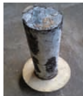
Fig. 4 The ingot of the ARCI sample which would be used for fabricating the prototype alternator
