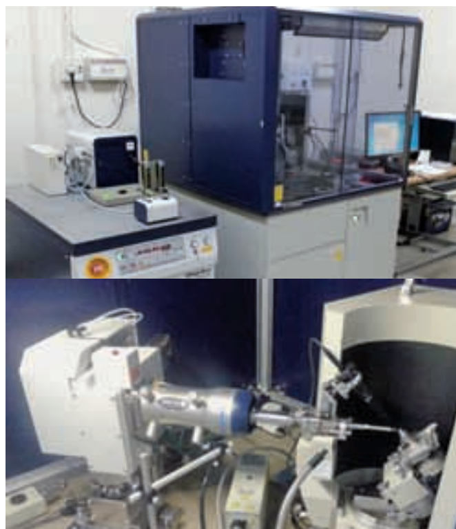
Fig. 1 (a) Rapid II D/MAX XRD system (b) setup showing the rotating anode, optics and detector behind the sample stage installed on the goniometer
