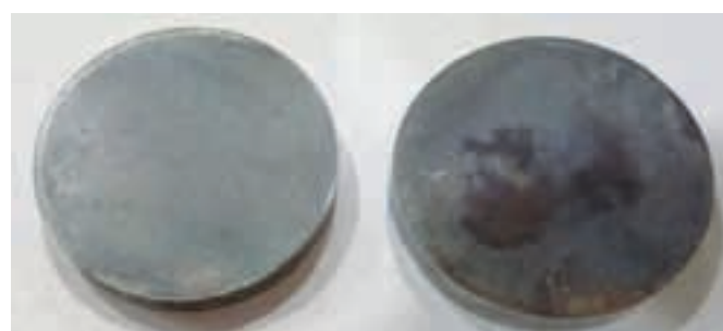
Fig. 2 Spark plasma sintered Cu and Ni doped PbTe samples
