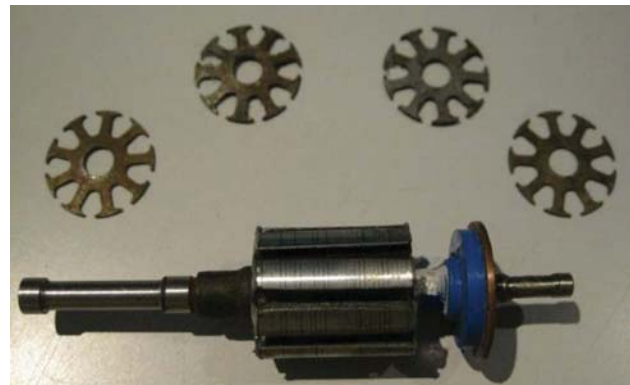
Fig. 2: A prototype motor assembled using the rotor fabricated from the Fe-P alloy synthesised at ARCI
