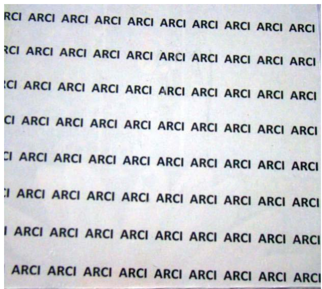
(b) Coated PC after taber testing
