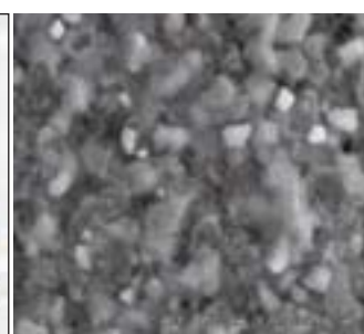
Fig. 3 Surface morphology of CIGS films after IPL treatment
