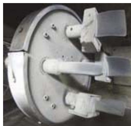
Fig.1 Manipulator used for TBC coating deposition on HPT Blade
