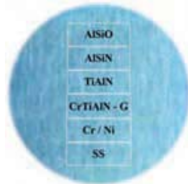
Fig.1 The schematic of Cr/G-CrTiAIN/TiAIN/AISiN/AISiO selective coating developed on SS-316 substrate (the background colour depicts the actual colour of the coating)
