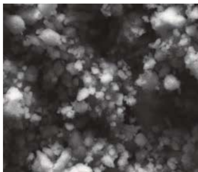
Fig. 2(a) SEM image of ( \text{Cu}_{10.5}\text{Zn}_{1.5}\text{Sb}_4\text{S}_{13} ) powder
