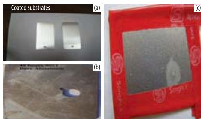
Fig. 1. Condition of the uncoated and coated test specimens after NaCl salt spray test (ASTM-117) a. Coated coupons, b. Uncoated & tested and c. Coated and tested.
