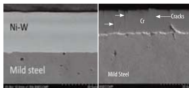
Fig. 1. SEM micrographs depicting Ni-W alloy and hard chrome coating cross section
