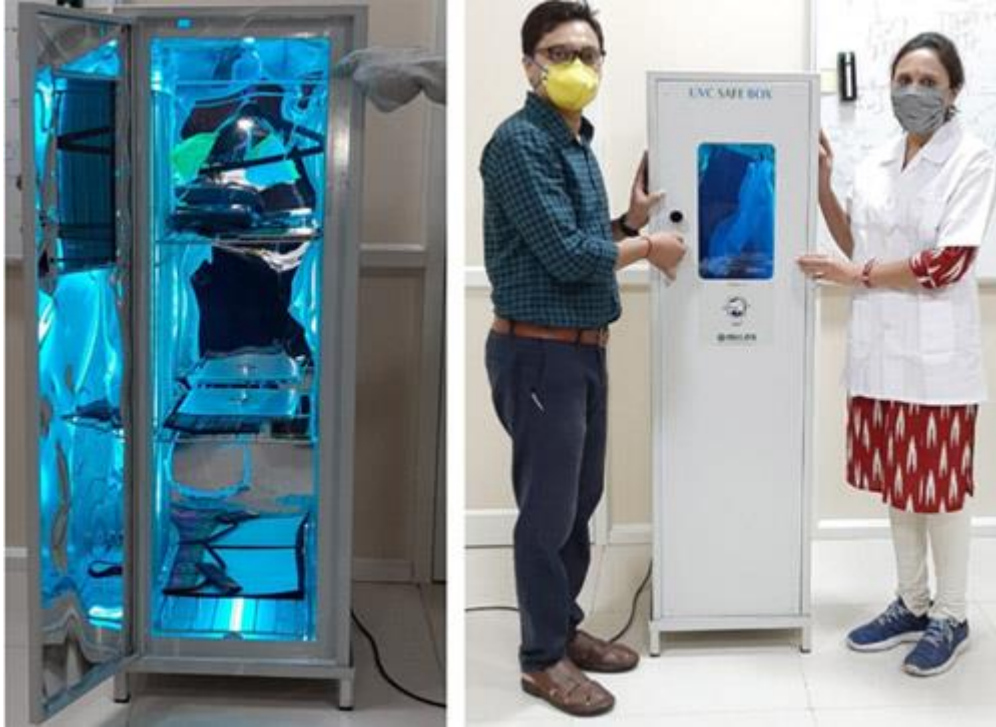
UVC-based multipurpose disinfection cabinet
