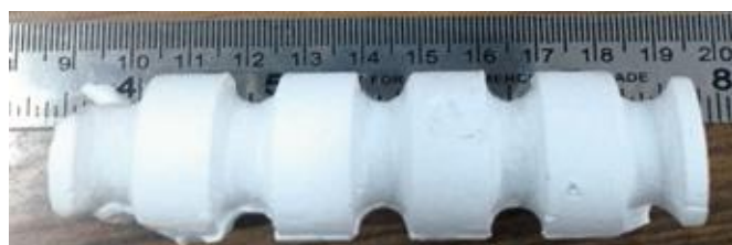
Fig. 3 Pressure cast \text{Al}_2\text{O}_3 spools sintered at 1600^\circ\text{C}
