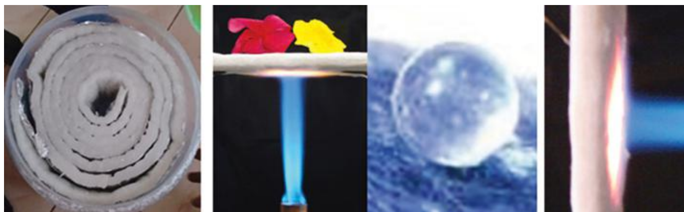
Fig. 1 Roll of silica aerogel flexible sheet, aerogel sheet protecting flowers from the blue flame, water drop-let on surface of sheet showing hydrophobic nature, fire resistance of the sheet
