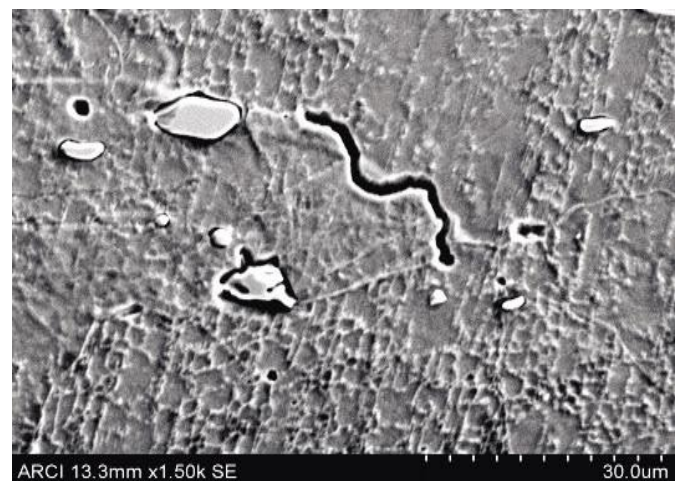
Fig. 3 Liquation crack near neck region of hybrid welds
