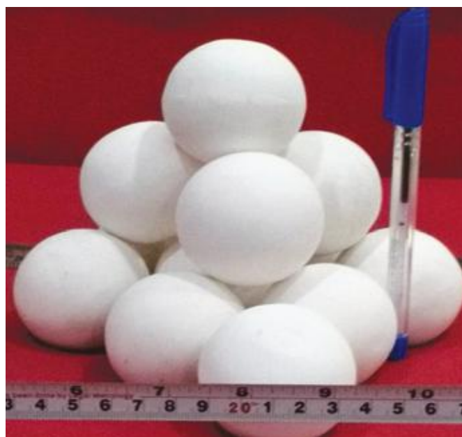
Fig.2 Pressure slip cast alumina grinding balls ( \text{Ø} 50 \text{ mm} ) sintered at 1600^\circ\text{C} to \approx 99\% density
