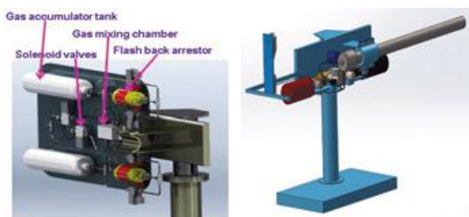
Fig.1 DSC gas control system and advanced detonation spray coating system
