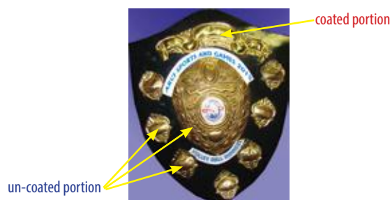
Fig. 3 Indicating the coated regions looking brand new while the uncoated region has faded
