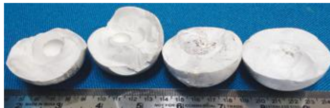
Fig.1 Sequential removal of hollow portion to reach full formation in half cut sintered alumina balls
