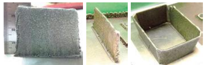
Fig. 3 Photographs showing as-build thin wall and rectangular geometries of satellite 6
