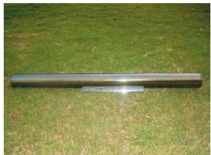
Fig. 3 Photograph of solar selective coated 1 m long SS tube
