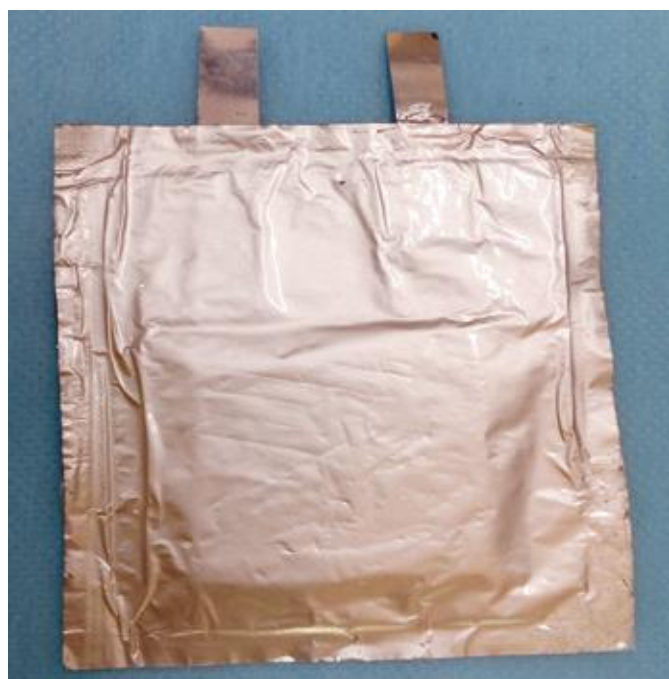
Fig. 1 Pouch cell assembly with \text{LiFePO}_4 cathode and graphite anode
