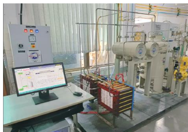
PEM Based ECMR for Hydrogen Generation
