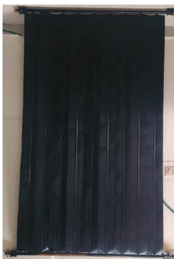
\text{CuMnNiO}_4 Spinel nanoparticles based absorber coated flat plate panel
