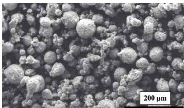
Fig.2 Scanning electron micrograph of spherical granules (Size 40-100 \mu\text{m} )
