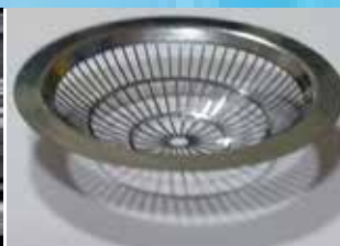
Control grid for pulsed microwave source fabricated using ultrafast laser
