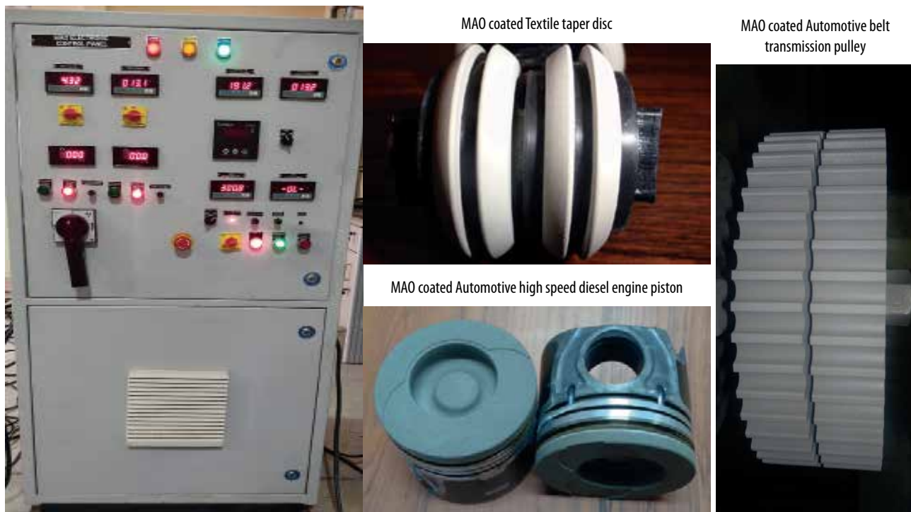
Fig. 8 Exclusively designed and custom built MAO control system being supplied to NIT-Tiruchirappalli in operation during its testing at ARCI
