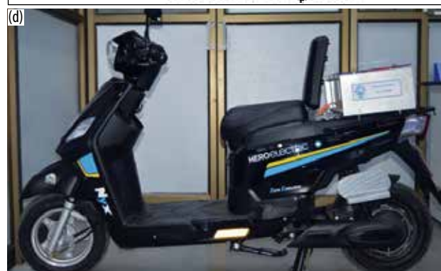
Fig. 1 (a) 3.2V, 18 Ah Li-ion prismatic cell and its charge/discharge characteristics at 0.3 C-rate (b) Cyclic performance of 18 Ah cell (c) 850 Wh battery pack with battery management system (BMS) (d) Demonstration of e-scooter with 850 Wh battery pack.
