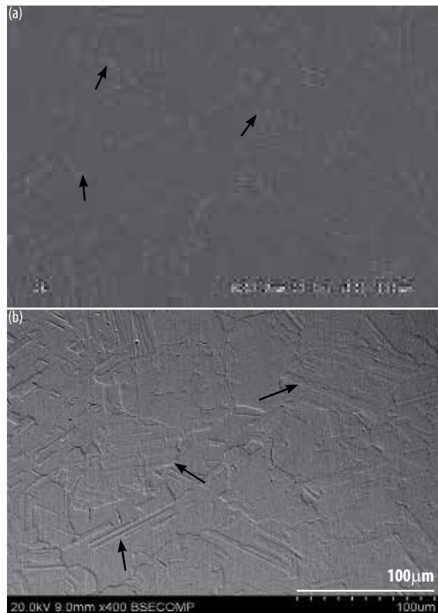
Fig. 5 Microstructure of ZnS samples (a) Vacuum sintered and (b) HIPed under identical temperature
