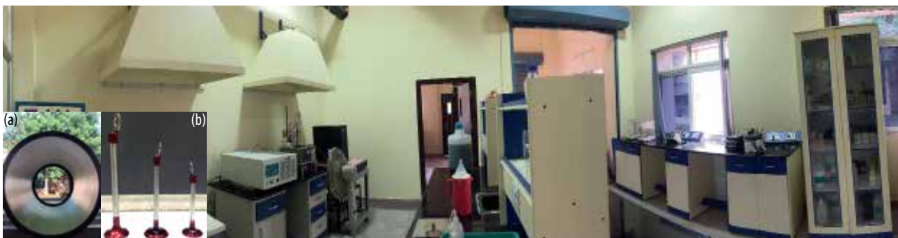
Pulsed Electro Deposited (PED) Coatings Lab Inset (a) PED coating inside engine cylinder liner (b) PED coating on engine exhaust valves
