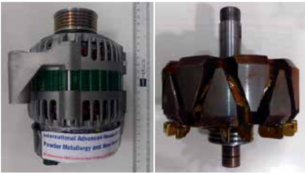
Prototype claw pole alternator and claw pole rotor developed using soft magnetic material
