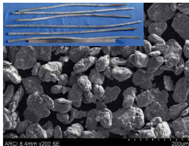
Fig. 6 SEM image of as-milled ODS RAFM-9Cr steel powder. Inset shows the extruded rods produced using the same powder
