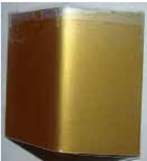
Chrome-free environmental friendly coating stack applied on AA2024 T3 alloy after 336 hrs of Salt Spray Test showing no corrosion at bent points
