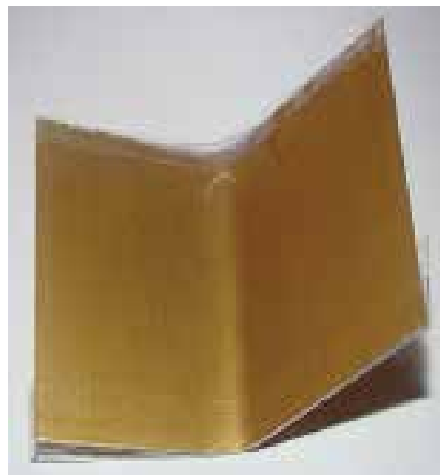
Chrome-free environmental friendly coating stack applied on AA2024 T3 alloy after 336 hrs of Salt Spray Test showing no corrosion at bent points
