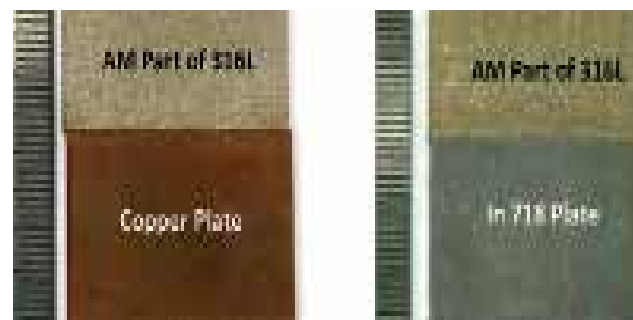
Fig. 3 Photographs of as built dissimilar metal parts
