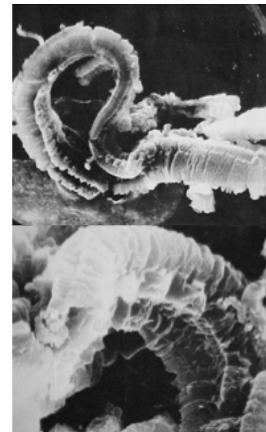
Fig. 1 SEM Micrograph of exfoliated graphite exhibiting worm structure
