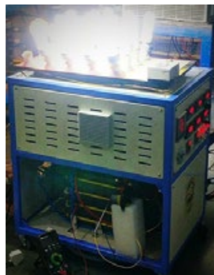
Fig. 1 Photograph during a virtual demonstration of the PEMFC system integrated with power condition to power AC lighting
