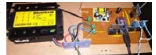
Fig. 3 Circuit for Auto switching of street lights
