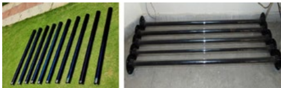
Fig. 5 Spectral selectivity of spinel nanocomposite based absorber coating on SS 304 substrate & images of multiple nos of 1m tubes and 2m prototype receiver assemblies developed for field validation
