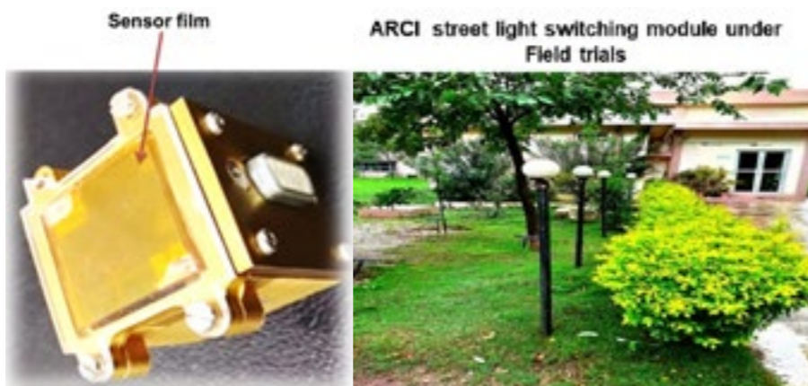
Fig.5 Device photograph of "circuit integrated photo-sensor" fully made in ARCI; Field trial carried out for ARCI fabricated solar light switching sensor in ARCI
