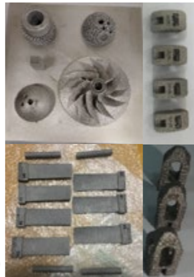
Fig. 2 Electron Beam Melting (EBM) for fabrication of various parts
