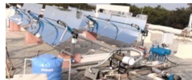
Parabolic test rig for validation of solar thermal components
