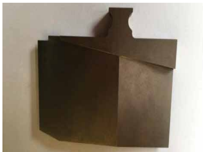
Fig. 3 Jet vane component of dimension 78 x 63 x 9 mm for commercial application machined out from the sheet shown in Fig. 2
