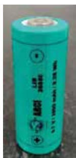
2.5 Ah NMC/ graphite cylindrical cell
