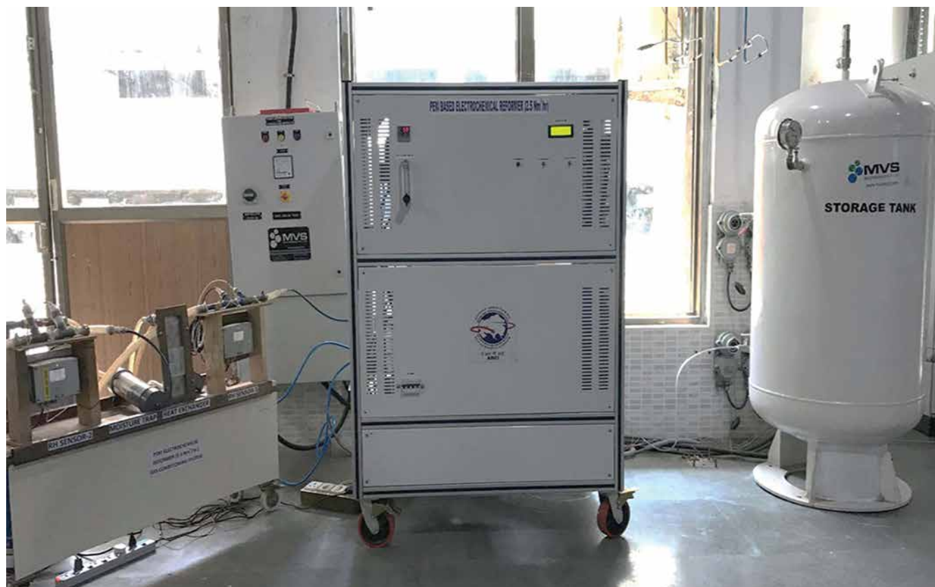
Fig. 1 Integrated ECMR unit of 2.5 Nm 3 /hr hydrogen production capacity with storage tank
