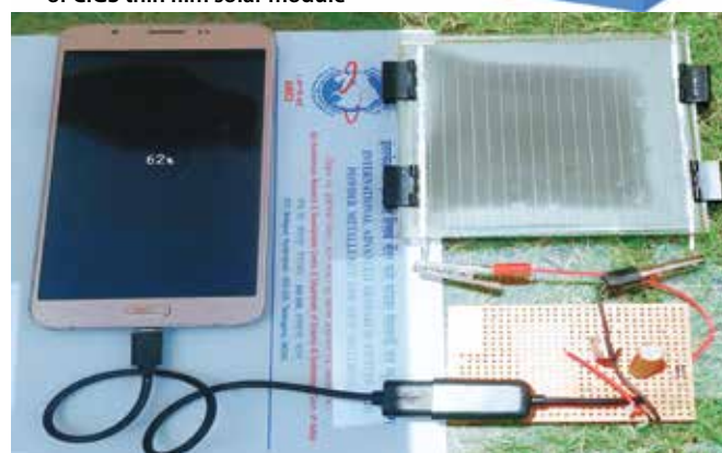
Fig. 3 Real time application demonstration of 100 cm 2 monolithically integrated prototype CIGS module for charging cell phone
