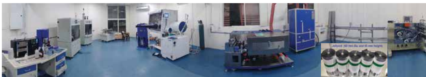
Semi pilot plant for the production of supercapacitors and photograph of jelly rolls as inset
