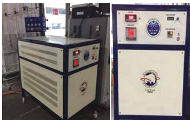
Fig. 1 The PEMFC system along with its balance of Plant components deployed at BARC
