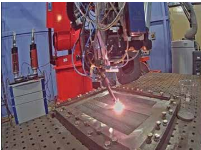
Laser Cladding of Burner Tip Plates
