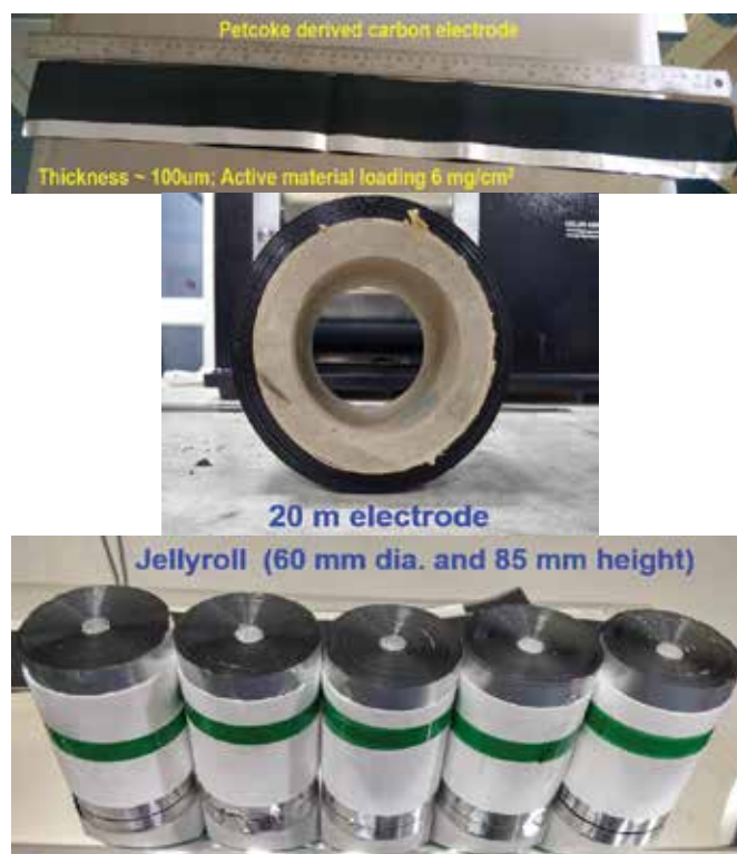
Fig. 2 Petcoke derived activated carbon electrodes and jelly rolls prepared at pliot scale supercapacitor facility
