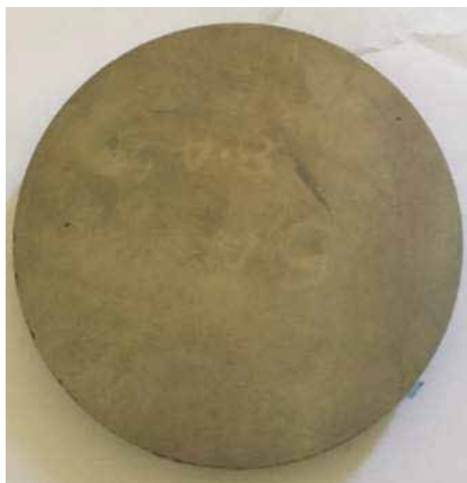
Fig. 2 High-strength, high-dense W-TaC sheets of 95 mm diameter fabricated by SPS
