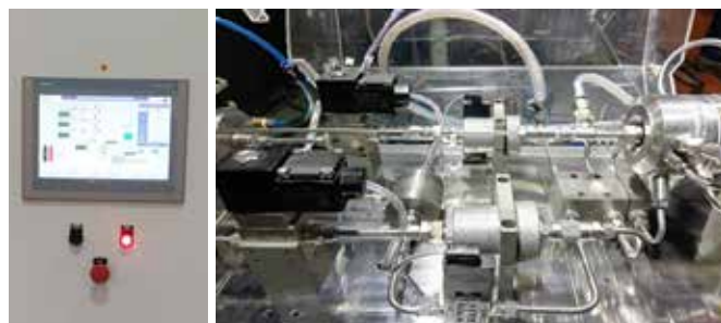
Fig.1 Advanced DSC system (Mark II) with HMI interface and electronic controllers
