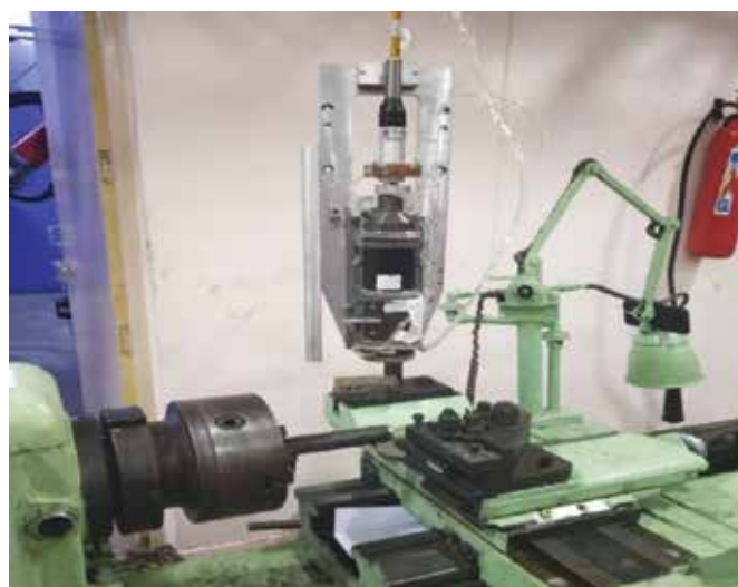
Fig. 2 Laser Assisted Machining setup at ARCI
