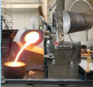
Vacuum Induction Melting (VIM) unit for alloys making
