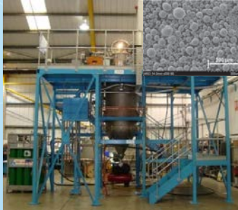
Inert Gas Atomization (IGA) for manufacturing AM grade powders
