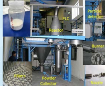
Flame Spray Pyrolysis unit for manufacturing oxide nanopowders
